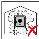
The inverter is designed to be dustproof (IP 66). In areas of high dust accumulation, dust deposits may collect on the cooling surfaces, and thus impair the thermal performance. Regular cleaning is required in this case, see chapter **Operation in dusty environments** on page 139. We therefore recommend not installing the device in areas and environments with high dust accumulation.
